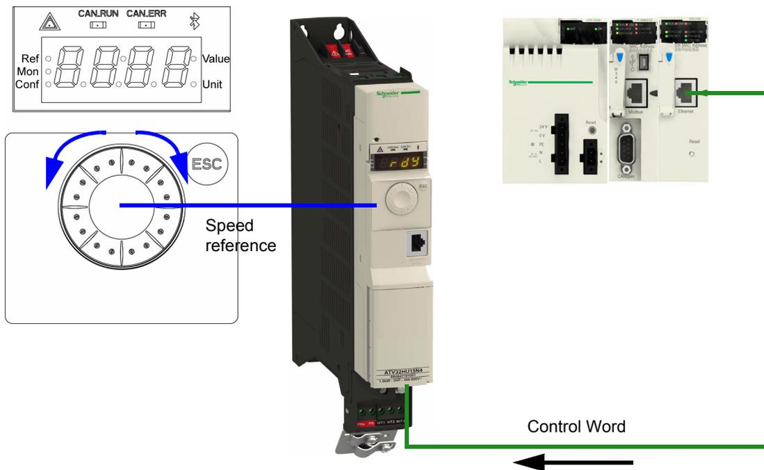
The drive is controlled from the communication (EtherNet) but the reference is adjusted on the local HMI. The control word comes from the controller and is written according to CiA402 profile.
