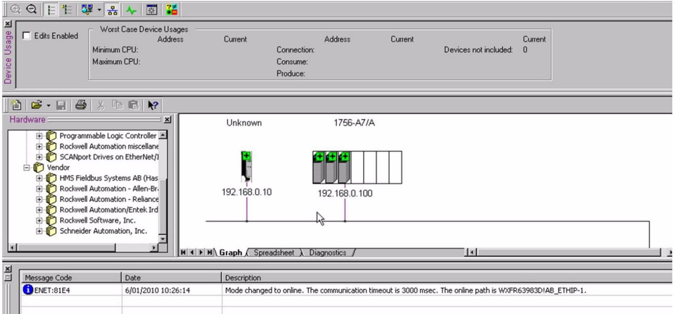
The VW3 A3 616 module is identified with the symbol: Generic Module. This identifier will be used later with tools such as the Class Instance editor.
