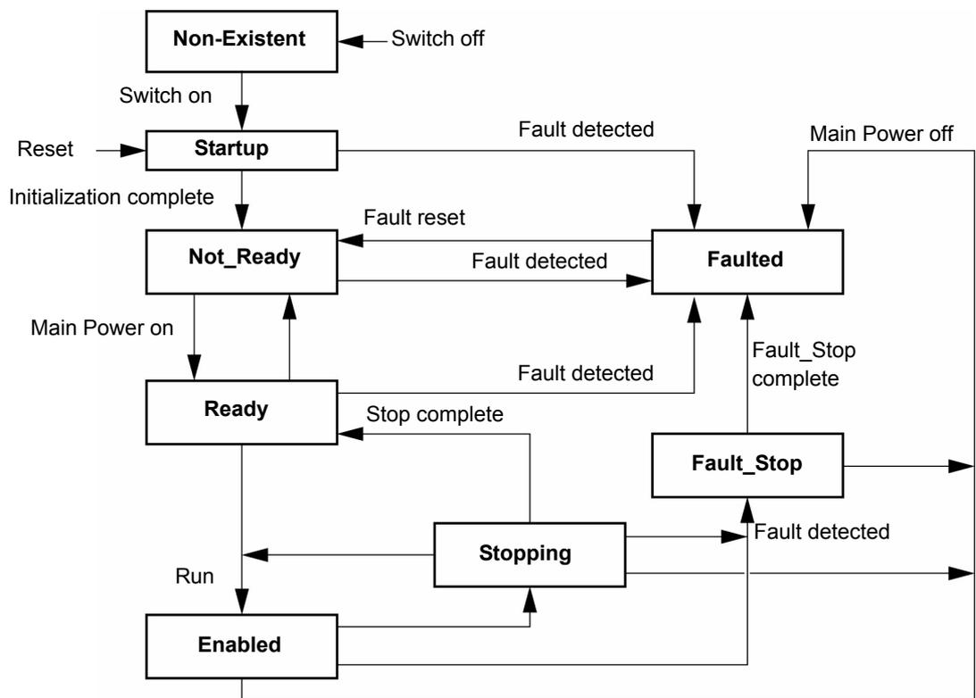
The Servo 3 drive state machine shall be supported as well. This state machine is already defined by D-SW.
