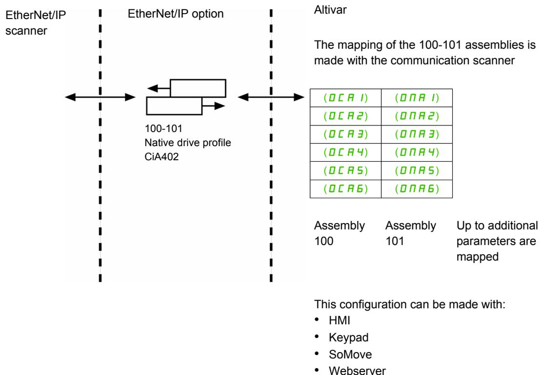
The size of the assembly (100, 101) is fixed and is equal to 6 words.
