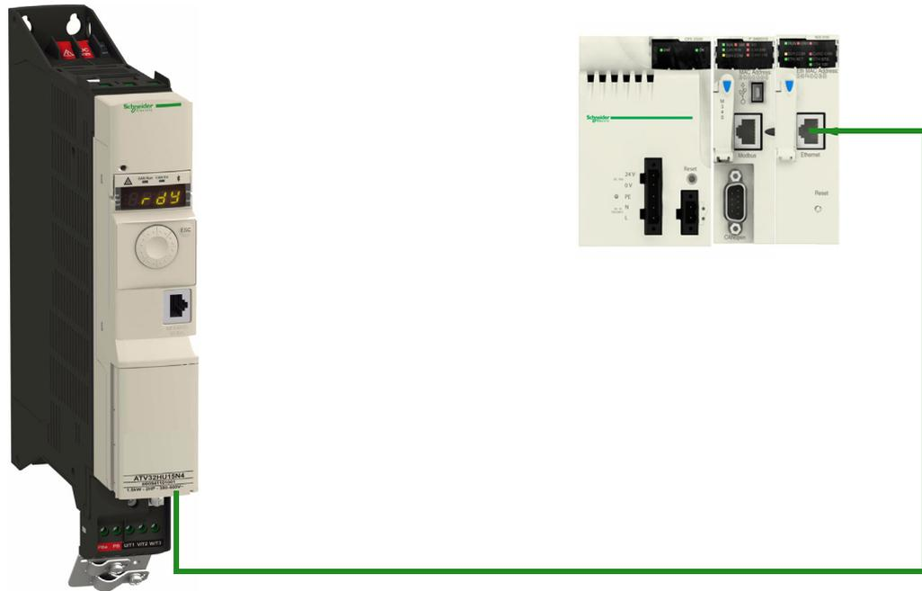
The ATV32 will be controlled through the option communication scanner by means of the I/O scanning service.
